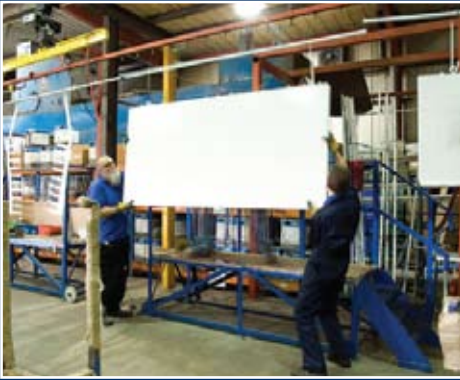
Door leaf manufactured from 1.5mm Zinc Coated Steel folded to a leaf depth of 66mm
